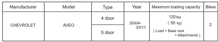
Maximum loading capacity is 55 kg (120 lbs) for this vehicle type.
